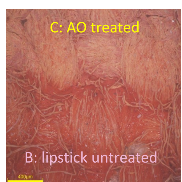
3D digital microscopy. Lipstick before (left) and after AO treatment
